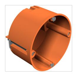
Cavity wall accessory socket. Dimensions to DIN 49073-1, for plate thickness 7–35 mm. Standard combination spacing 71 mm, option for continuous wiring using connection support for combinations between accessory sockets and accessory connection sockets, 8 break-out openings for NYM cables, data cables and pipes  $\varnothing$  20 mm, accessory sockets can also be used as connection sockets to VDE 0606-1 with double bolt fastening and screw-on cover, protection rating IP20.
